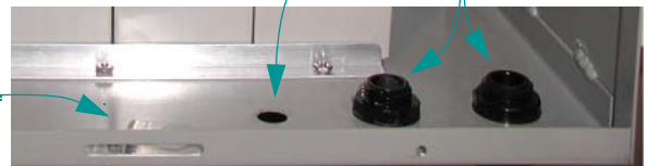
ac inputs / outputs are via 12 mm (1/2") diameter knockouts, (shown are optional liquid-tight cable glands and an optional third hole for OEM use)
